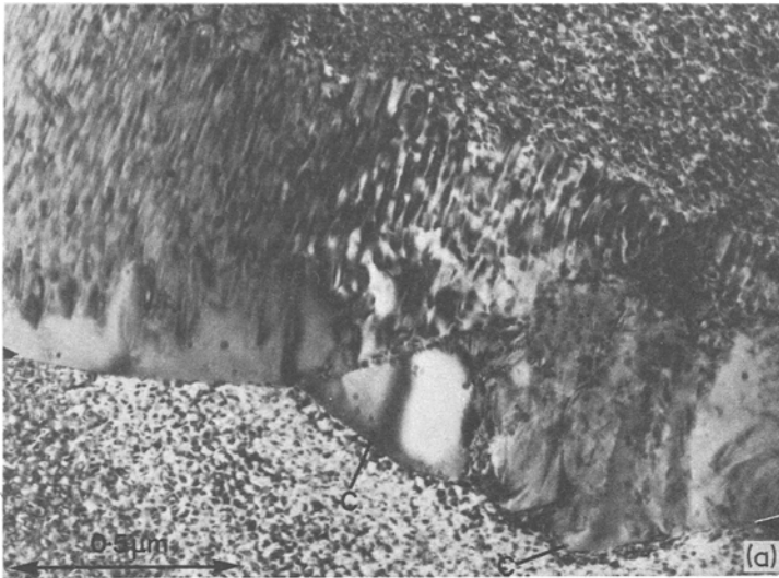
Figure 7 Alloy 3, standard two-stage heat treatment. The lamellar part of the colonies shown here contains only \gamma and \gamma' , and carbide is seen at the incoherent reaction interface. (a) A perturbation in the lamellar aggregate is seen around the "blocky" carbide particles (indicated by C). (b) The same colony is seen here in a different contrast condition, in which the carbide particles are in dark contrast. (c) There is a continuous film of carbide along the incoherent interface of this colony (arrowed), and also some "blocky" particles.
