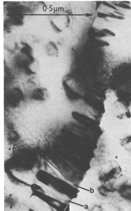
Figure 1 Alloy 1, standard 3-stage heat treatment. This shows two small cellular colonies on a grain boundary (arrowed), with one colony nucleated on each grain. In the lower colony, nucleated on the left-hand grain, laths of \gamma' (a, b) which have grown on a prior \gamma' particle (c) are indicated. The carbide laths are in dark contrast.
