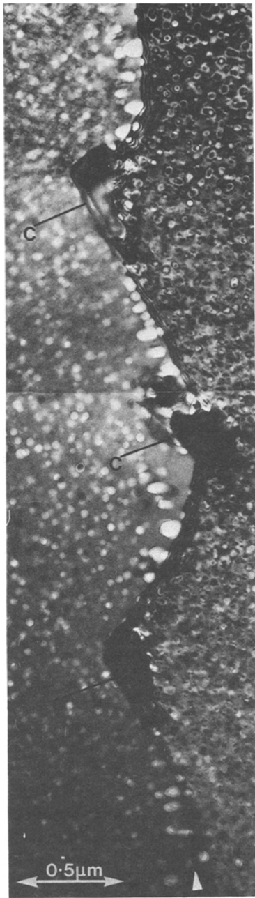
Figure 6 Alloy 2, 2 h at 1050° C + 2 h at 850° C. The cellular precipitate here is all nucleated on the same grain. The boundary is slightly bowed in between the large M_{23}C_6 carbide particles (arrowed), and elongated \gamma' particles are seen. The shape of the carbide particles is typical of nuclei for cellular precipitates by the conventional mechanism.
